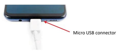
Connect the power charger cable to the provisioned device. The device will usually fully charge in approximately 2 hours.
