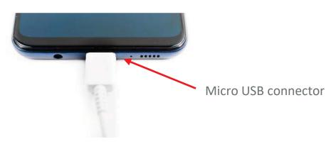
Connect the power charger cable to the provisioned device. The device will usually fully charge in approximately 2 hours.
